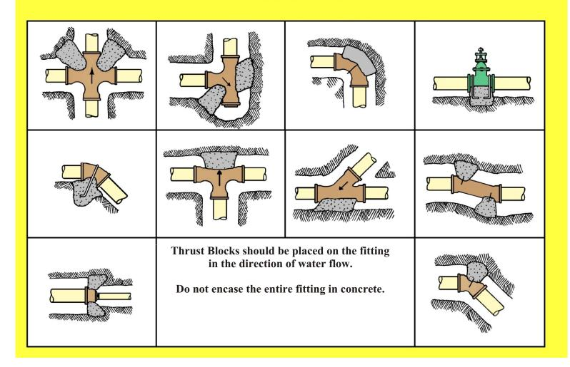
Thrust blocking should be used on all gasket joint pipe and fittings since there are great thrusts developed whenever there are changes in direction in the pipeline, dead ends, pipe sizes and valves. These thrusts can blow the joints apart creating big messes.
