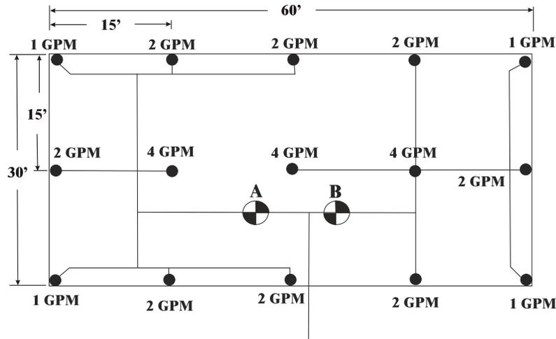
In the above example there are 2 zones with 16 G.P.M. each for a total of 32 G.P.M. The total area is 60' x 30' or 1800 sq ft. The heads are spaces 15' x 15' or 225 sq ft.
